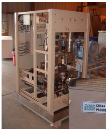
Chena Hot Springs Electrolyzer, used to generate 6kg of Hydrogen per day
